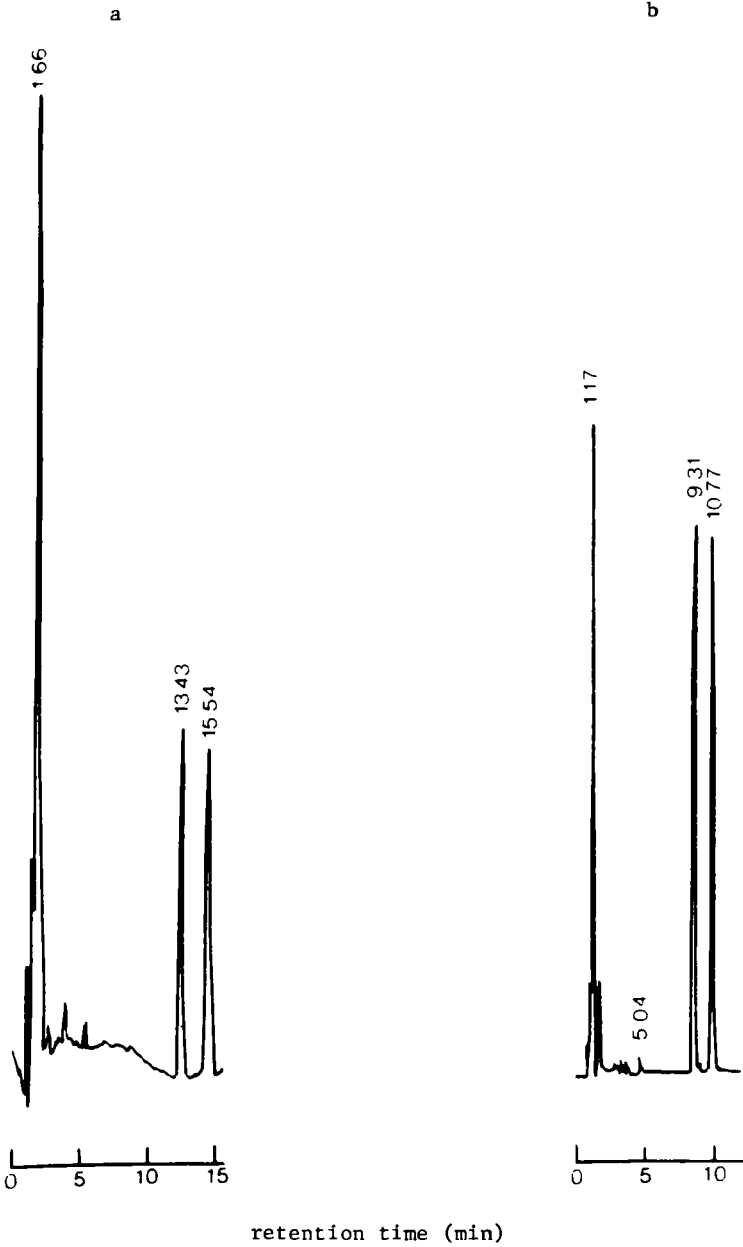
Figure 2. Separation of cis - and trans - Permethrin by HPLC. Column: Regis ODS-2, 5 \mu m Solvent System: CH 3 CN:H 2 O = 70:30 a) Flow Rate: 1.0 mL/min b) Flow Rate: 1.5 mL/min
